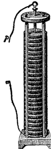
A sketch of the original voltaic pile invented by Alessandro Volta
